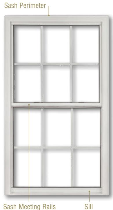
The Air Leakage (AL) rating pertains to air infiltration that occurs through the window unit itself. It is expressed as the equivalent cubic feet of air passing through a square foot of window area per minute. Air leakage typically may occur through the window assembly components, such as the sash perimeter, sash meeting rails and sill.
